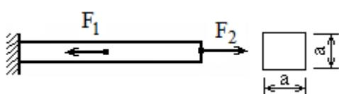
$F_1 = 10 \text{ кН}$ ,  $F_2 = 30 \text{ кН}$ ,  $\sigma_T = 300 \text{ МПа}$ ,
